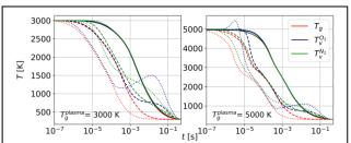
**Fig. 1**. Evolution of different temperatures as a function of axial distance.  $T_g^{plasma}$ ,  $T_g$ ,  $T_v^{O_2}$  and  $T_v^{N_2}$  represent the gas temperature in the plasma and quenching regions, as well as the vibrational temperatures of  $O_2$  and  $N_2$  in the quenching region. Solid, dashed, and dotted lines correspond to cooling enhanced by factors of 10, 100, and 500, respectively.
